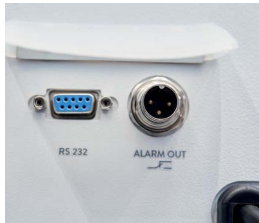
Standard-issue RS-232 interface and alarm contact
